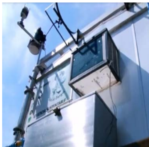
Fig. 2 (a) Subsystem modules of the weather station, and (b) Weather station installed on the roof of a sustainable home
