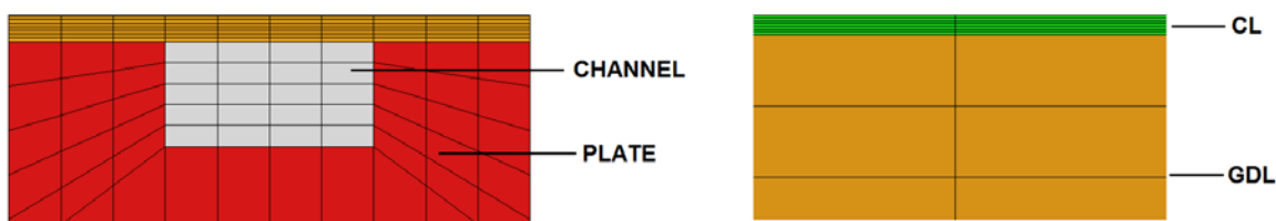
Fig. 2. Mesh visualization and components of PEM electrolyzer model.
